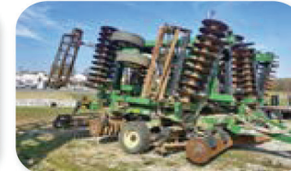
2019 McFarlane IC5140 , 40' Incite VT Tool, 20.75" Frt., 20.25" Rear, Hyd. Angle Blades, Chopper Reel $67,500
